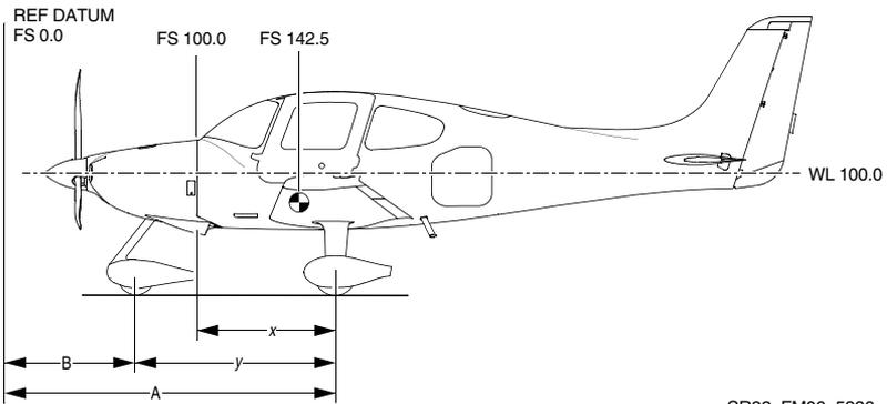
Basic empty weight, moment, and center of gravity are provided in inches aft of datum, where 0 inches datum is 100.0 inches forward of the cabin firewall. CG can also be expressed in terms of its location as a percentage of the airplane Mean Aerodynamic Cord (MAC) using the following formula:
